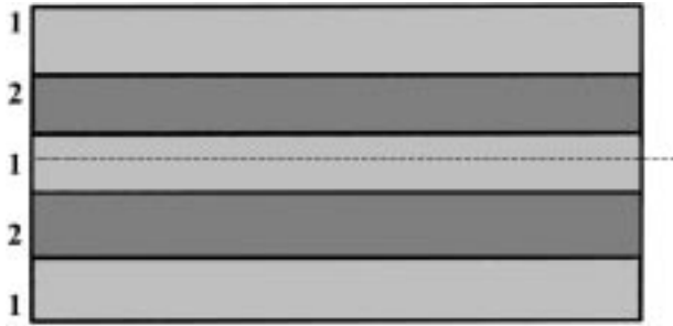
Fig. 1. Two-component layered composite: 1—layers of the first component including two external (outside) layers; 2—layers of the second component (internal).
