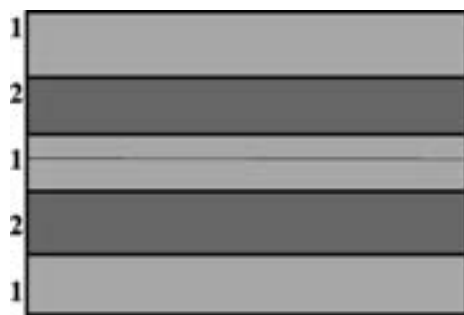
Fig. 1. Two-component layered composite: (1) layers of the first component including two external (outside) layers; (2) layers of the second component (internal).
