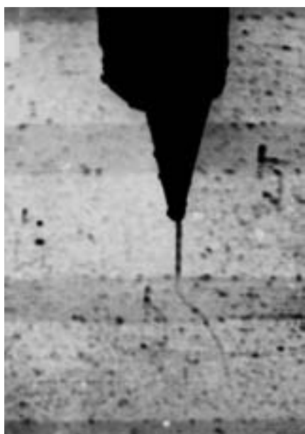
Fig. 4. Optical photograph of layered specimen with typical notch tip.
